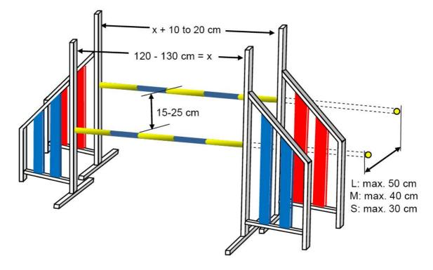
Two single hurdles (as above) can be placed together to form a spread hurdle. The poles are placed in ascending order with a difference in height of 15 to 25 cm. The length of the pole on the back hurdle must be 10 to 20 cm longer than the pole on the front hurdle.
