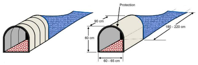
It must have an entrance of rigid or semi-rigid construction with a depth of 90 cm.
