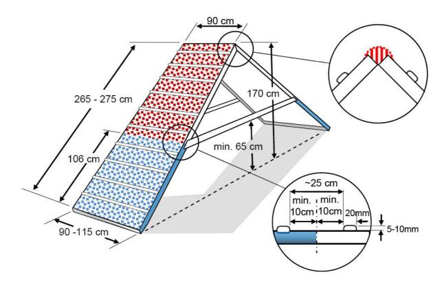
Height: The apex of the two ramps must be 170 cm from the ground for all dogs.
