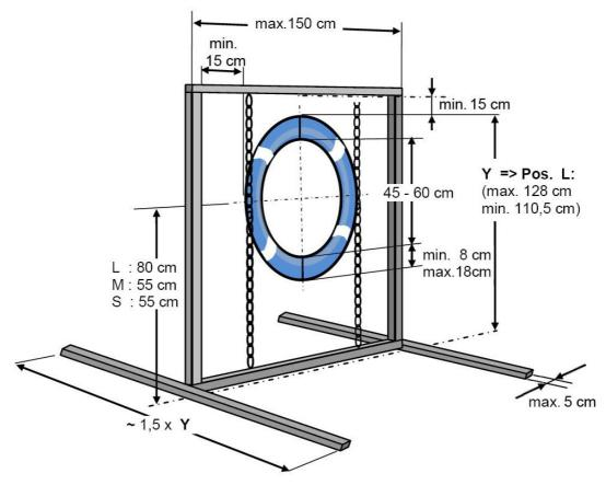
The tyre must be adjustable in height (chains or rope), fixed or rigid attachments are not allowed. The tyre must be able to break away into 2 to 4 parts when a force equivalent to a weight of 8 kg is exerted on it.
