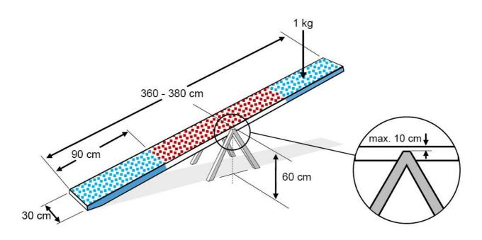
Height: 60 cm measured from the ground to the top of the plank at the central pivot point. The pivot point of the see-saw must not be more than 10 cm beneath the top of the plank.
