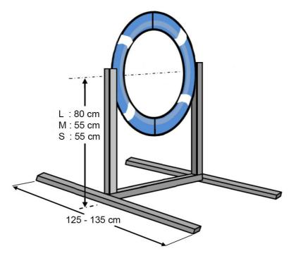
The tyre must have a consistent shape, constructed using an impact absorbing material. The tyre is fixed into position (height) by two uprights on either side of the tyre. The construction must provide sufficient stability to ensure that the obstacle is not tipped over too easily. The uprights must not protrude above the top of the tyre. There should be no beam across the top.
