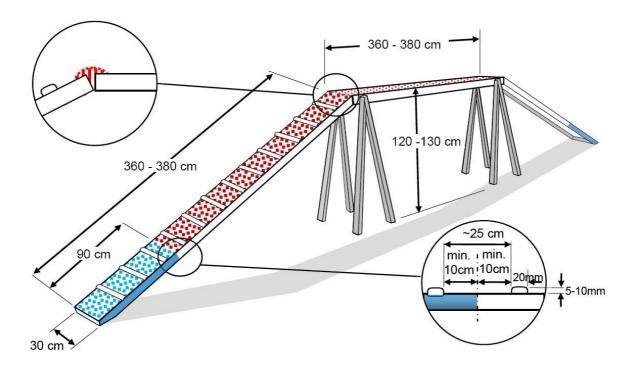
Height: minimum 120 cm – maximum 130 cm Plank and ramp length: minimum 360 cm – maximum 380 cm Plank and ramp width: 30 cm
